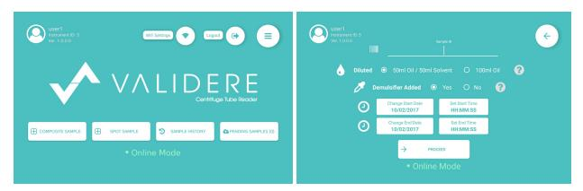
**Step-by-step instructions and automatic results** - the CTR's intuitive user interface walks the operator through each step of the procedure and then reports the result. There is no need to write down water content or enter results manually.
